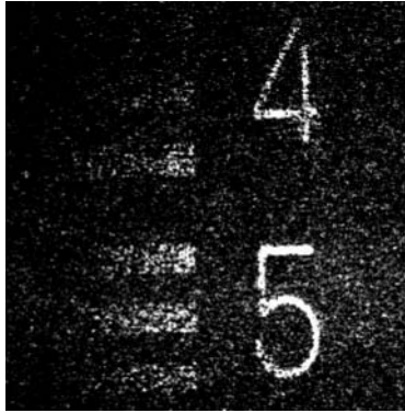
Fig. 28. Portion of an Air Force bar-target imaged through nine scattering mean free paths using low-coherence holographic time-gating in a photorefractive polymer in the near infra-red (800 nm)
