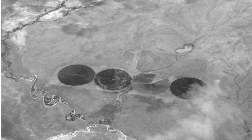
Figure 6-6 These circles are irrigated fields in western Texas. Water is supplied by a well at the center of each circle.
