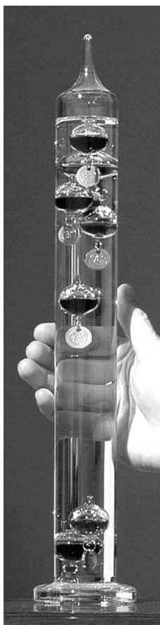
Figure 1-7 In a Galileo thermometer, as the water inside the tube becomes warmer and less dense, more of the weighted glass spheres sink to the bottom. The tag on the lowest sphere that floats indicates the approximate temperature.
