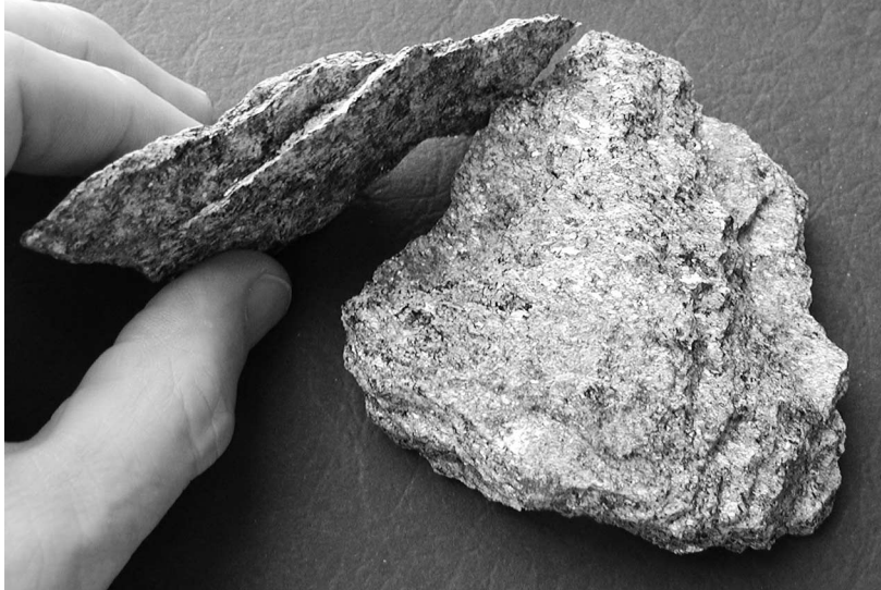
Figure 5-12 The way schist breaks in layers is a result of the parallel growth of mica crystals. This parallel alignment of mineral crystals is called foliation.
