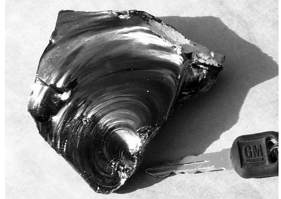
Figure 5-6 The glassy texture of obsidian (volcanic glass) indicates that it cooled very quickly.
