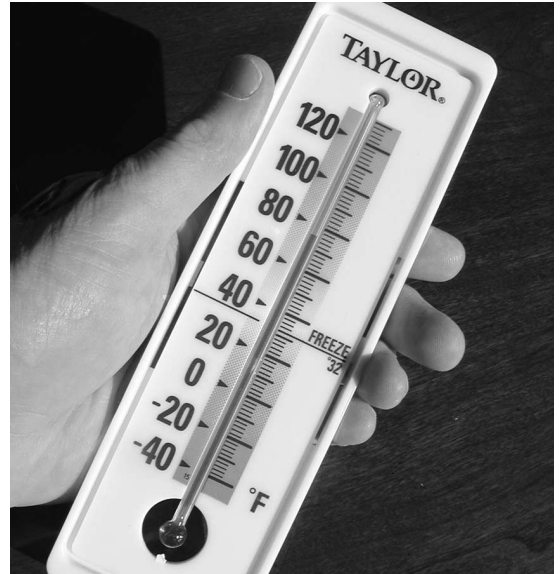
Figure 19-2 A thermometer contains colored alcohol in a glass bulb at its bottom. The alcohol expands or contracts in the tube, registering changes in temperature.
