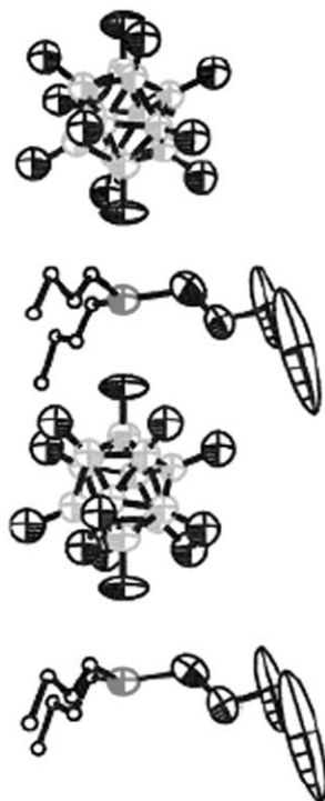
FIG. 12. Part of an infinite column of alternating cations and anions as a detail of the crystal structure of [n\text{-Bu}_3\text{Sn}^+][\text{CB}_{11}\text{Me}_{12}] . Thermal ellipsoids are drawn at 50% probability level. Hydrogen atoms and one component of the disordered butyl groups are omitted for clarity, Sn and B atoms are gray and C atoms are black. (Reprinted with permission from Ref. 68. Copyright 2000, American Chemical Society.)
