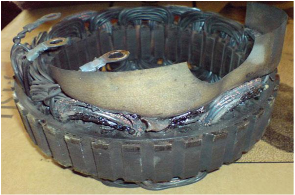
1.2-rasm.Stator cho'lg'aming shikastlanishi
