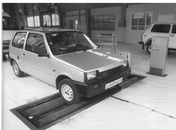
6.1-rasm. Rolikli STM-8000 rusumli stendda avtomobil tormozini diagnostikalash.
