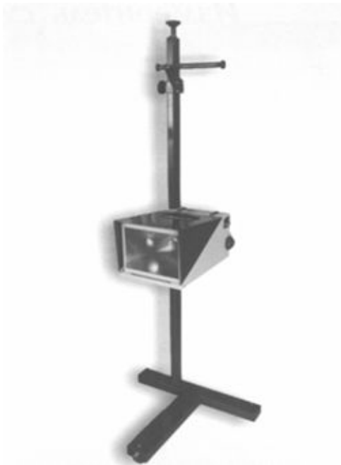
5.6-rasm. Avtomobil faralarining parametrlarini diagnostikalash uchun IPF-01 jihozi (a) va tekshirish jarayoni (b)
