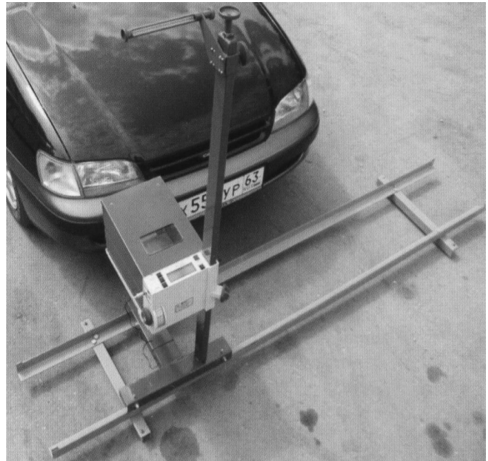
5.6-rasm. Avtomobil faralarining parametrlarini diagnostikalash uchun IPF-01 jihozi (a) va tekshirish jarayoni (b)
