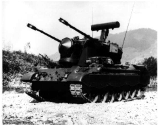
Figure R29 Flakpanzer anti-aircraft tank system. The K a -band fire control tracker shares the forward antenna with a longer range X-band tracker, whose transmitter also serves the target acquisition radar at the rear of the turret.
