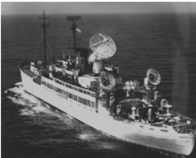
Figure R35 Range instrumentation ship (RCA photo).
