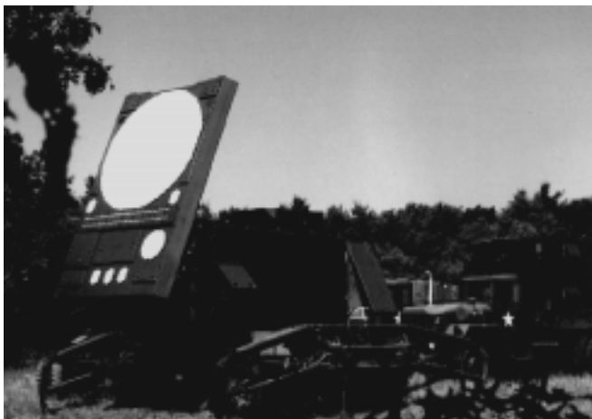
Figure R41 AN/MPQ-53 Patriot multifunction array radar (Raytheon photo).
