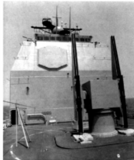
Figure R42 AN/SPY-1 Aegis multifunction array radar (from Brookner, 1988, Fig. 3.A.1-3, p. 257).
