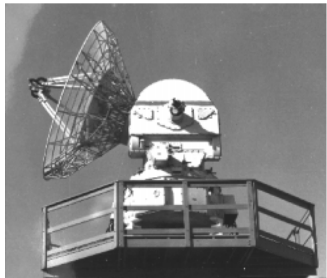
Figure R33 AN/FPS-16 instrumentation radar (RCA photo).
