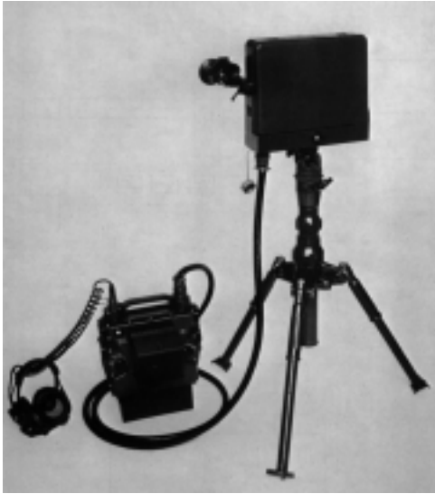
Figure R51 Typical man-portable personnel detection radar for battlefield use.
