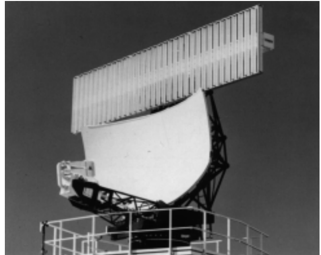
Figure R9 ASR-10SS radar antenna (Raytheon Company photo).
