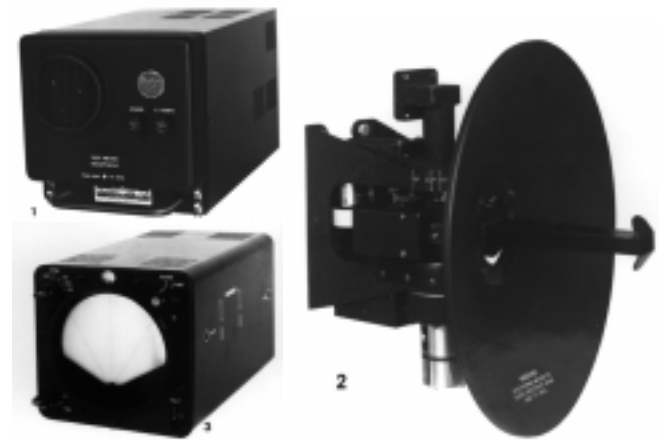
Figure R6 AVQ-55 weather-avoidance radar components: (1) transmitter-receiver unit, (2) antenna, and (3) display (RCA photograph).
