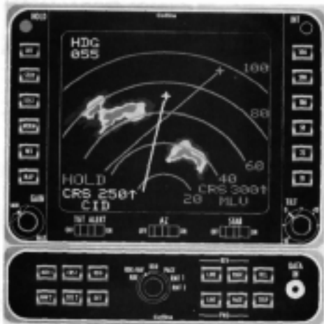
Figure R7 Cockpit display of WXR-300 weather-avoidance radar data (Collins photograph).
