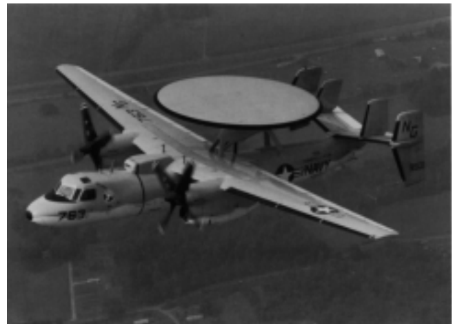
Figure R82 E-2C AEW aircraft with rotodome antenna.
