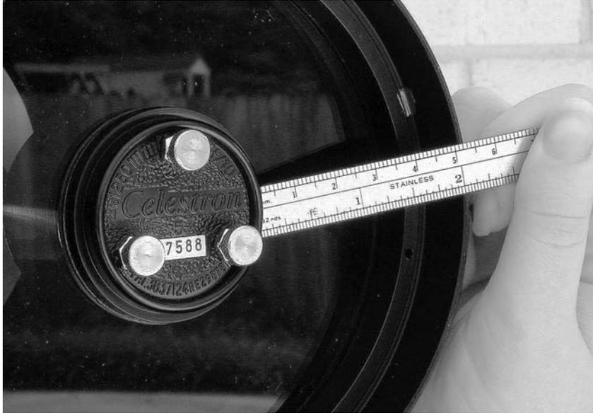
Figure 5.10. Using a ruler to check that the secondary holder is centered. Note thumbscrews installed in place of original collimation screws.
