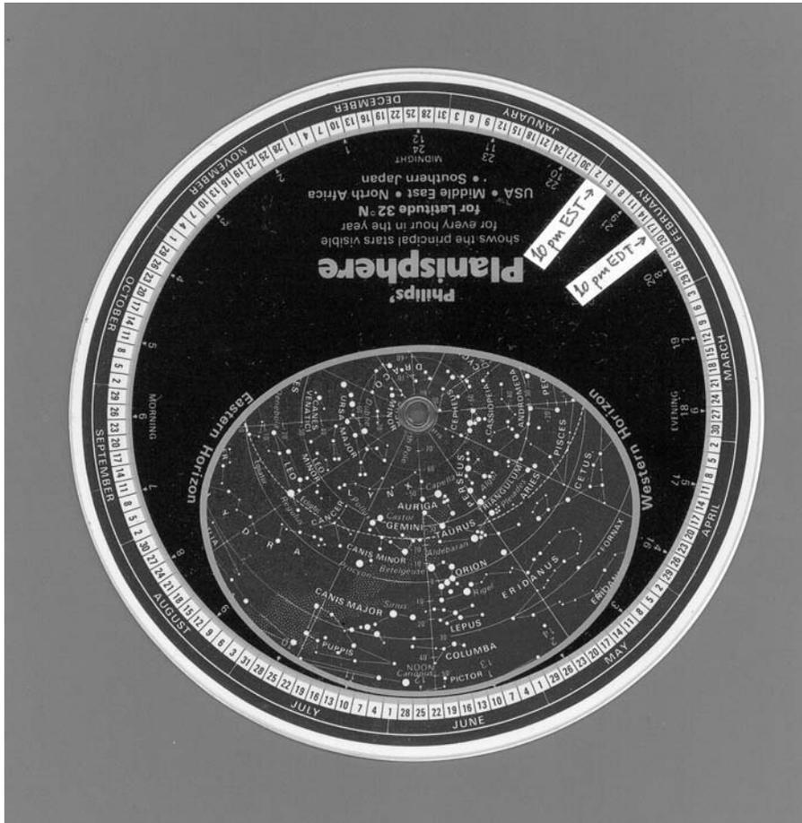
Figure 2.6. The author’s well-worn planisphere, with handmade labels showing the difference between local mean time and zone time (winter and summer). Local horizon could also be drawn in.
