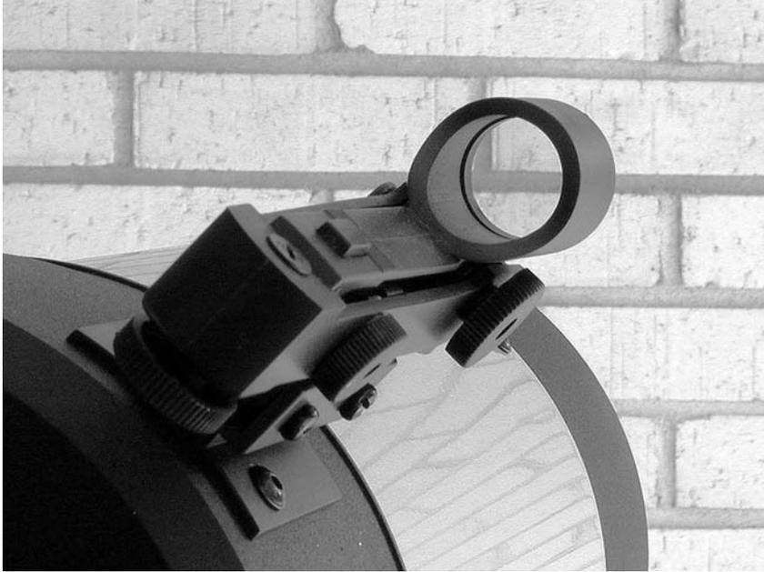
Figure 6.12. Nonmagnifying LED finder on Celestron NexStar 5. Seen through its window, a red spot appears superimposed on the sky.
