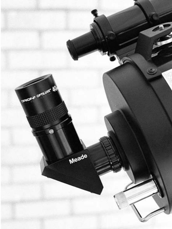
Figure 6.5. This Meade 2-inch mirror diagonal attaches directly to the back of the telescope. An adapter for  $1\frac{1}{4}$ -inch eyepieces is provided with it.
