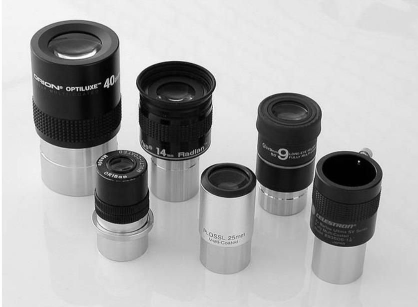
Figure 6.1. Eyepieces. Back row, left to right: 40-mm König (an Erfle variant) in a 2-inch barrel; 14-mm Radian and 9-mm Lanthanum LV in 1 $\frac{1}{4}$ -inch barrels. Front row: 18-mm orthoscopic with parafocalizing ring held in place by set screw; 25-mm Plössl; Celestron Ultima 2 $\times$  Barlow lens.
