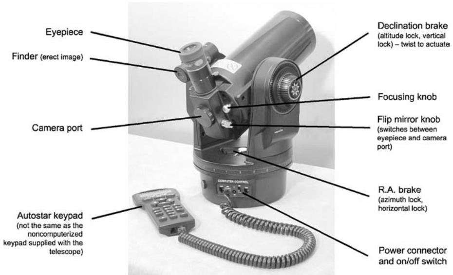
Figure 12.1. Main parts of the Meade ETX-90. Other ETX and LX90 telescopes are similar.
