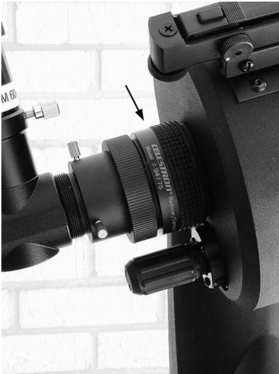
Figure 6.9. Focal reducer attaches to telescope ahead of diagonal and eyepiece.
