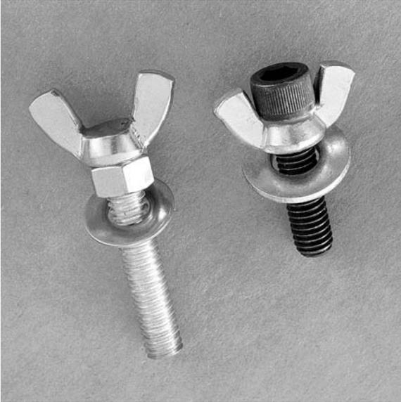
Figure 4.10. Homemade thumbscrews. Left: wing nut, ordinary nut, and threaded rod. Right: wing nut and bolt. High-strength epoxy holds the wing nuts in place.
