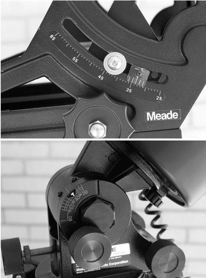
Figure 4.5. Scales on the wedge or tripod indicate correct inclination for your latitude. Meade Superwedge (top); Meade ETX-90 field tripod (bottom).
