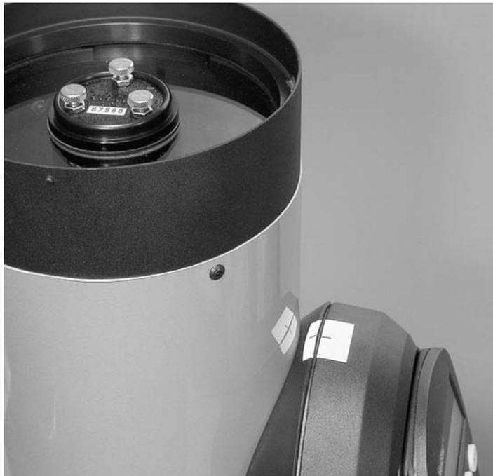
Figure 11.4. Pieces of tape, suitably marked, can help you level the NexStar tube (top) or point it away from its base for polar alignment (bottom). Exact positions can be found with a bubble level, then marked.
