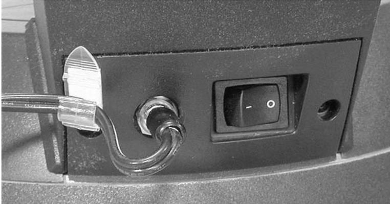
Figure 11.2. A stick-on telephone-wire clip helps keep the power cord from pulling out as the telescope rotates.
