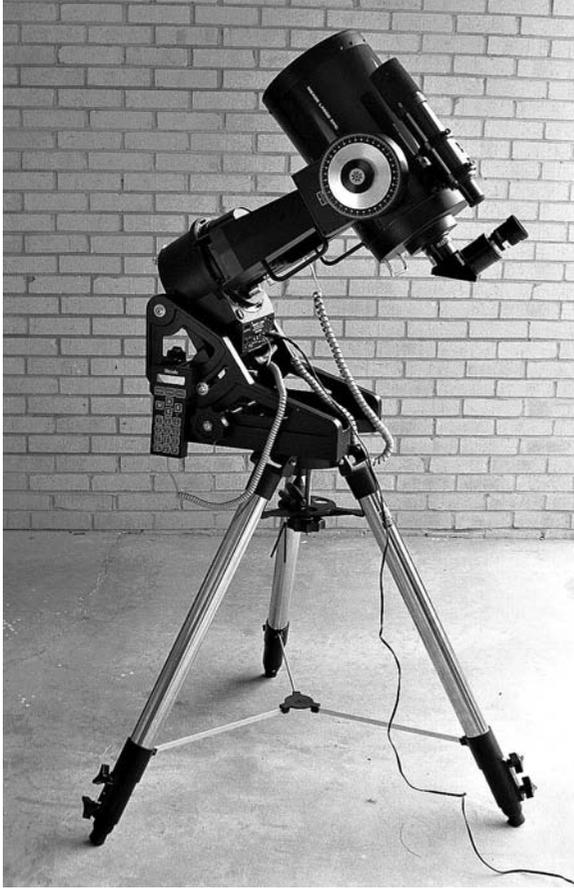
Figure 4.1. Meade LX200 telescope equatorially mounted on Meade Superwedge and field tripod. Compare Figure 3.1.
