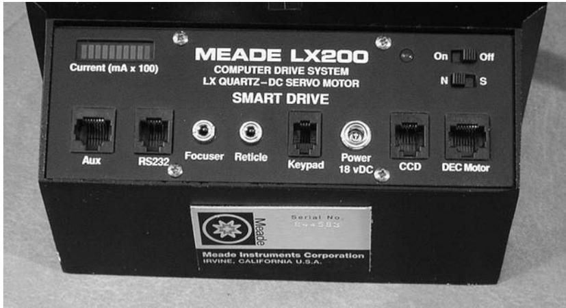
Figure 10.2. The LX200 connector panel. Bargraph display at upper left is ammeter, showing current consumed by telescope.
