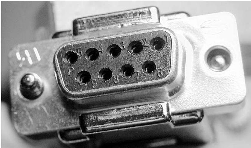
Figure 10.9. Pin numbers are imprinted on serial port connectors for positive identification.
