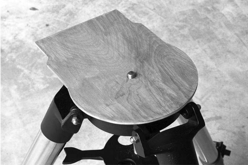
Figure 3.7. A homemade template makes it much easier to center the LX200 on its tripod. This one is plywood, but cardboard would work just as well.
