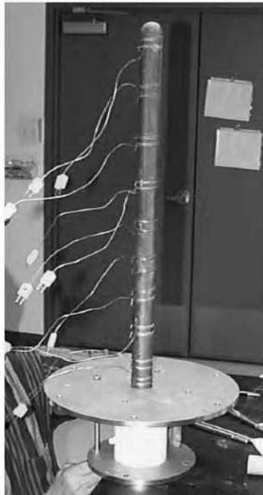
FIGURE 4.13 A schematic and a prototype of a SiC bayonet H 2 SO 4 vaporizer/decomposer.
